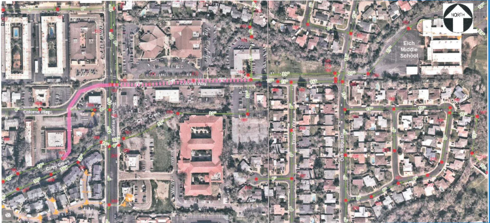
Coloma Way Alignment - Diversion from Cirby Truck A to Truck B (dash = upsized, solid = new, x = abandon)
